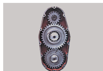
Gear driven, final drive
