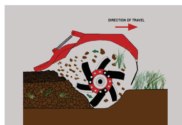
Reverse rotation models bury clods & debris
